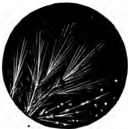
GLYKO-CHOLATE OF SODA FROM OX-BILE, after two days' crystallization. At the lower part of the figure the crystals are melting into drops, from the evaporation of the ether and absorption of moisture.
